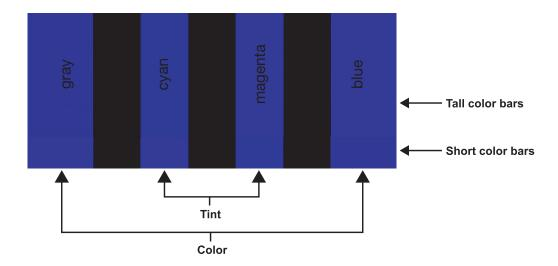
**Tint:** Tint or "hue" is essentially the ratio of red to green in the color portion of the image. When tint is decreased, the image appears redder; when it is increased the image appears greener. To set the tint, select Tint and press **ENTER** or **SELECT**. While looking at the color bar pattern through a blue filter, adjust the tint level until the cyan and magenta color bars (on either side of the green bar) appear to be a single shade of blue.
